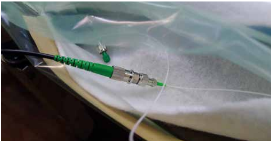
Connector plug (FC-APC) for optical fibres (photo: T. Fildhuth, ITKE)
