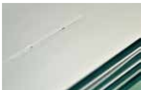
Fibre-optical sensor fixed inside the four-layered glass laminate using a transparent adhesive (glue length = 60 mm) (photo: A. Ehret, ITKE)
