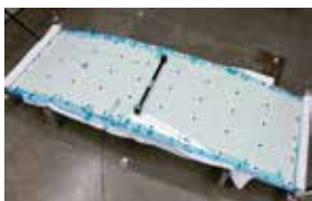
Cold bent glass fixed on its bending mould after lamination (photo: T. Fildhuth, ITKE)
