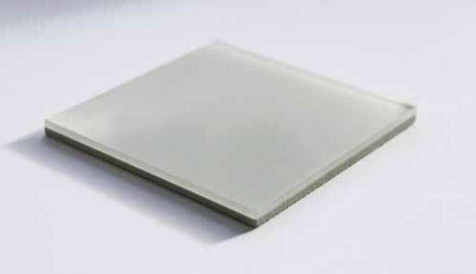
FKV-VH-Element (© Alina F. L. Joachim) Sample for ventilated façade with FRP (fibre-reinforced polymer) (© Alina F. L. Joachim)
