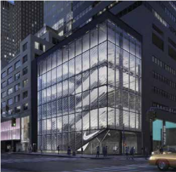
Nike Flagship Façade – Carved and Slumped Insulating Glass Units
