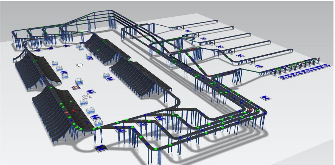
Model of the distribution centre created using Siemens Plant Simulation. The software is used to create a digital twin of an entire operation, enabling users to run tests, gather data and ultimately create innovation in an environment with no risk.
