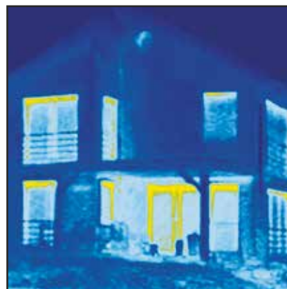
Thermal image of a detached house with Ködispace insulation glazing. The good thermal insulation is recognizable from the absence of red areas.
